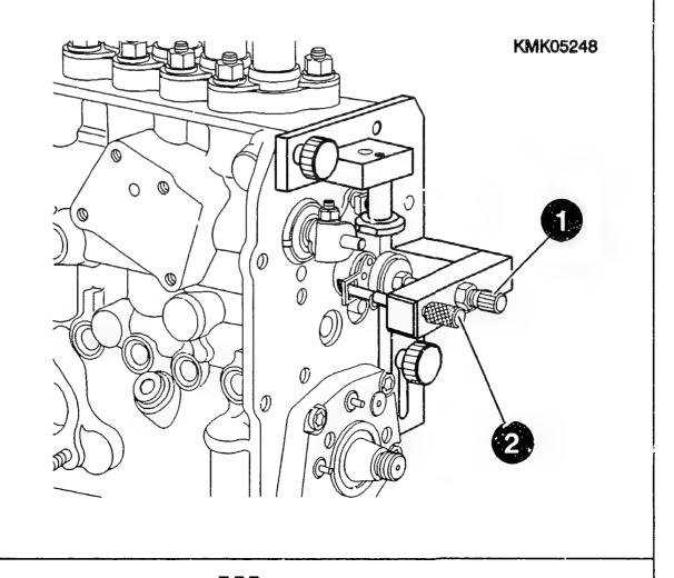
Checking position of RPS shortcircuiting ring: Before attaching setting device, stop bracket for control lever of prestroke shaft may have to be removed for space reasons. Support setting device at positioning pin at top right of pump housing and screw into the appropriate tapped holes in the housing using the two kr.urled screws. Set control rod with adjusting screw (1) to roughly (estimate) half travel. Check position of ring with measuring rod (2).
